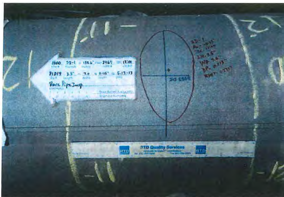
Figure 5. External Appearance of the Flash Welded Pipe Seam on Line 1600
