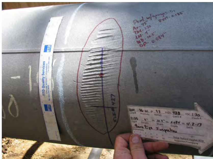
Figure 10. Prior Mechanical Damage Discovered on Line 1600
