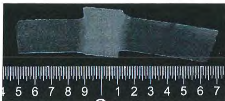
Figure 6. Typical Flash Welded Seam Cross Section, ca. 1946
